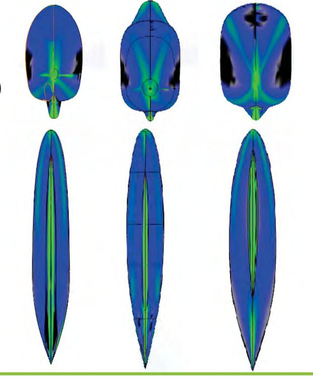
The selected design solution resulted competitive with these reference prototypes in terms of drag and, as a consequence, in terms of power required to travel at a given speed.
