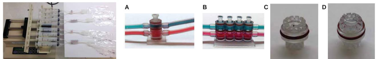
Fig.4 Experimental setup: A) flux mix for one cell B) flux mix for 4-cells-array C) insert without scaffold D) insert with scaffold
