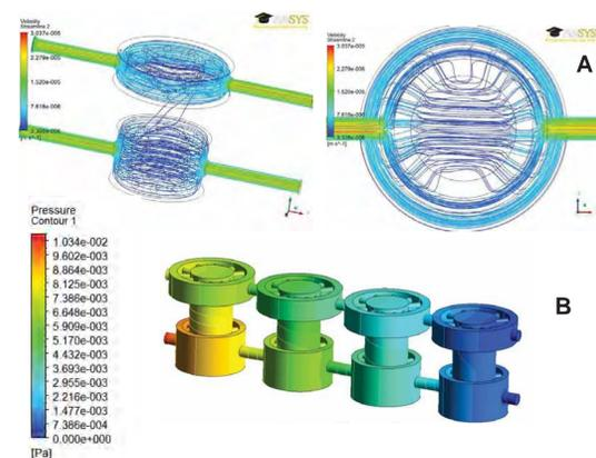
Fig.5 A) flux stream lines B) mass flow distribution
