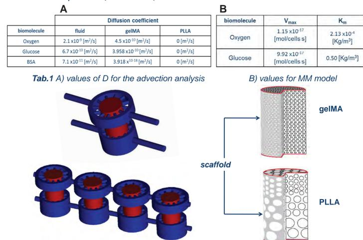
Fig.2 Single and 4 array configurations (left) and sketch of the 2 types of scaffold (right).
