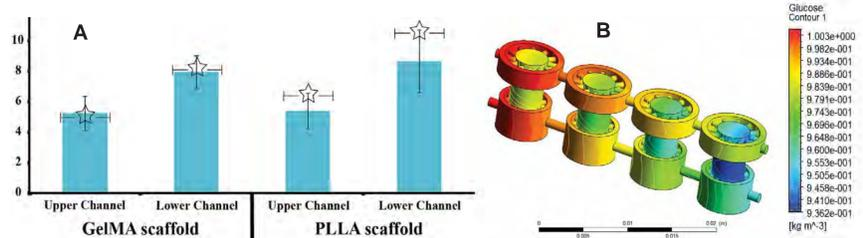
Fig.7 A) glucose consumption: numerical vs experimental data B) consumption evolution in one cell and along the 4-cells-array
