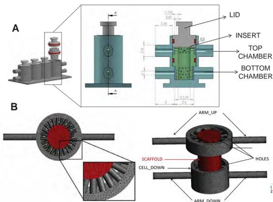
Fig.1 A) CAD model (dimensions in mm) B) mesh.
