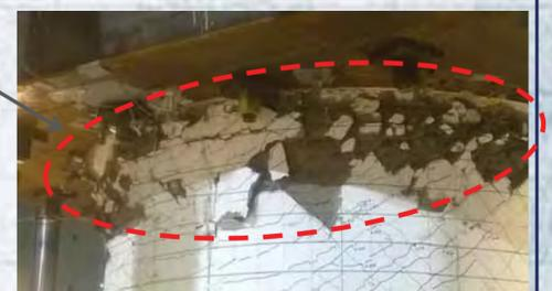
Figure 7. Sliding shear failure at interface (Credits: Stocchi).
