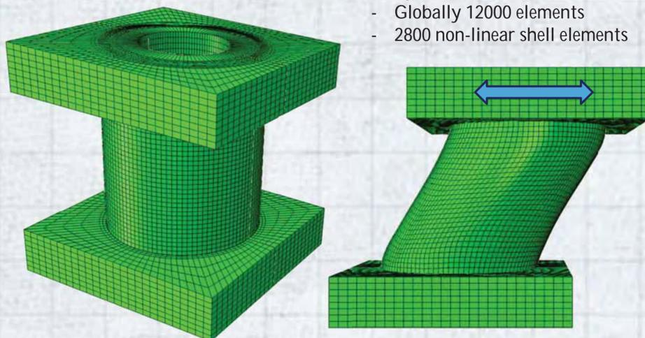
Figure 3. Numerical model for undefromed and deformed shape.
