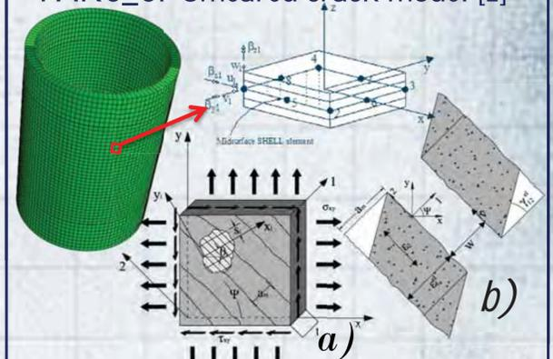
Figure 4. FEM model and a) reinforced concrete element subjected to plane stress state, b) kinematic quantities
