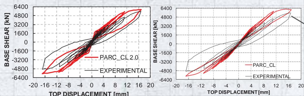
Figure 6. Base shear vs. top displacement respectively for the plastic and the secant model.
