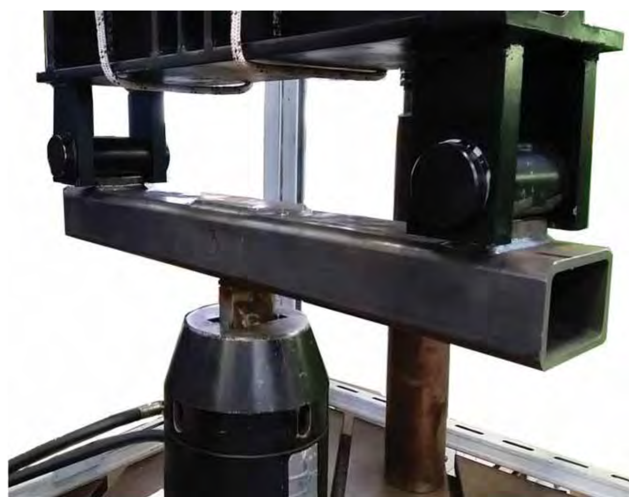
Welded joint clamped in the fatigue machine.
