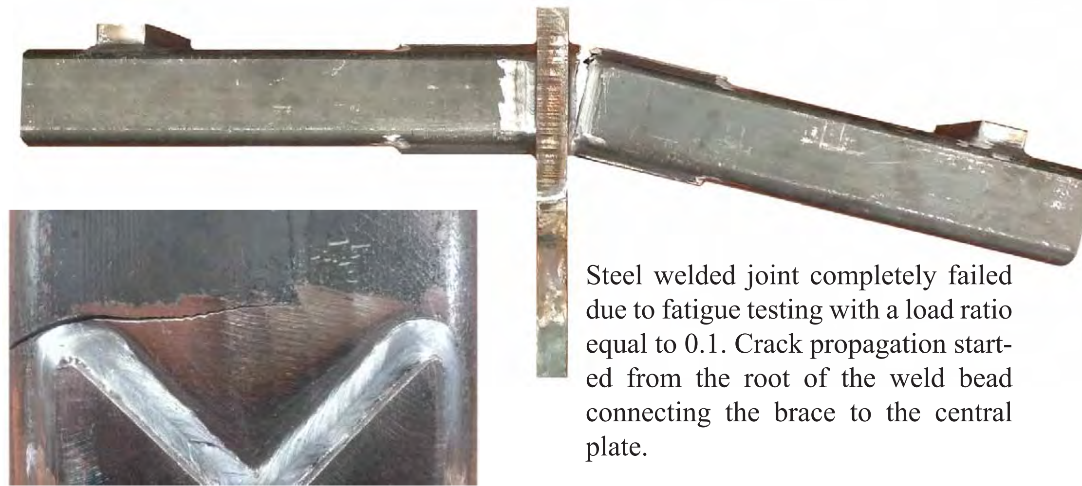
Fatigue crack at weld toe.
